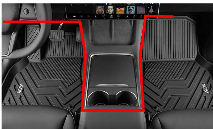
(3) .拆下马鞍两侧饰板，左侧前后门把手线材按照上图走线至副驾驶控制盒放置位置，控制盒隐藏在饰板里面 Remove the decorative plates on both sides of the saddle, and route the left front and rear door handle wire to the position of the copilot control box according to the figure above. The control box is hidden inside the decorative plate
