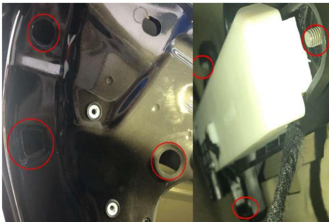
(9).取出上图三颗螺丝,拆下原车把手 Take out the three screws in the picture above and remove the original handlebar
