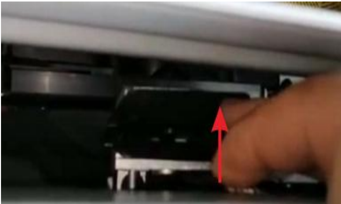
(5).玻璃有卡扣需要同时拿螺丝刀拨住才能取出玻璃 The glass has a buckle. You need to hold the screwdriver at the same time to remove the glass
