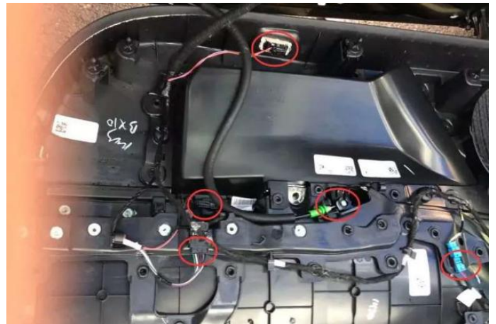
(4). 把与盖板相连的插线拔下 拿下盖板 Remove the plug wire connected to the cover plate and remove the cover plate
