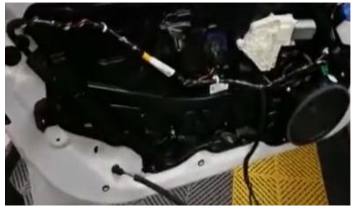
(6).拔掉与饰板相连的插头 Remove the plug connected to the trim plate
