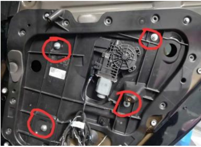
(7).除了图中红圈内四颗螺丝外，全部取下 Remove all screws from the fastening trim plate
