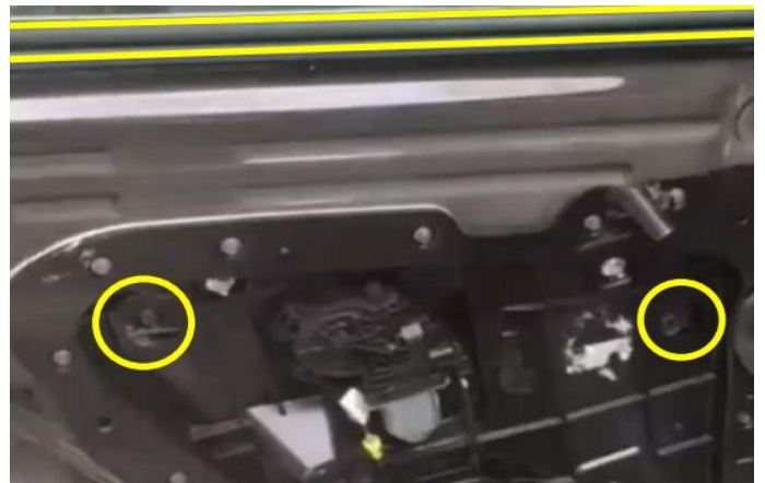
(6). 拿出标示处胶条和胶塞把两圆圈内玻璃螺丝拧出就可以直接把玻璃拿出来了 Take out the rubber strip and rubber plug at the mark and unscrew the glass screws inside the two circles to take out the glass directly
