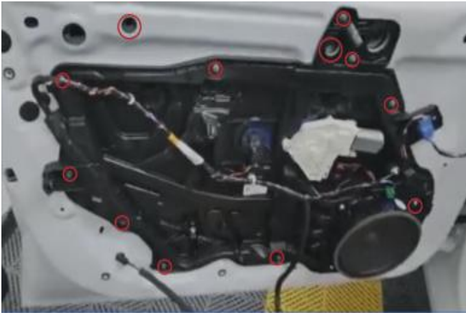
(5).拔掉所有插头取下标记的所有螺丝拿下饰板 Unplug all plugs, remove all marked screws and remove the trim plate
