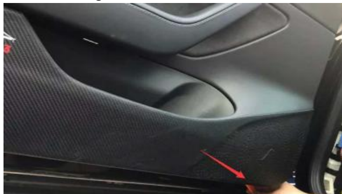
(2).用撬刀撬右下角 卸下门饰板 Pry the lower right corner with a pry knife to remove the door trim panel
