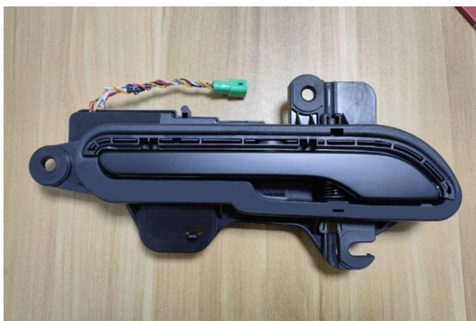
(11).将第二代把手安装到车上,用原车螺丝固定 Install the second generation handle on the car and secure it with the original car screws
