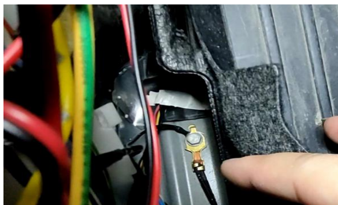
(4) .在主驾驶脚踏旁边接地线。接好之后测试把手，把手工作正常即可恢复车门饰板 Ground wire next to main driver's foot. After connecting the handle, test the handle to restore the door trim panel when it works normally
