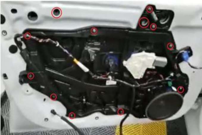
(7).取下标记的所有螺丝，拿下饰板 Remove all screws from the mark and remove the trim plate
