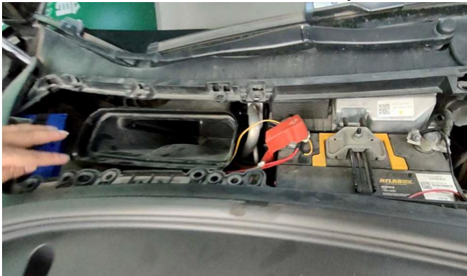
(1) .在前盖电池取电，左边找孔穿线至副驾驶 Connect the cable to the battery in the front cover, find a hole on the left side and thread the cable to the co-pilot
