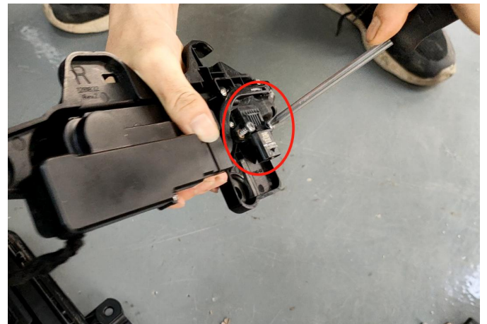
(10).将原车上的信号器拆装到相对应的电动把手上,用原车螺丝固定 Disassemble the signal on the original vehicle to the corresponding electric handle and fix it with the original vehicle screw
