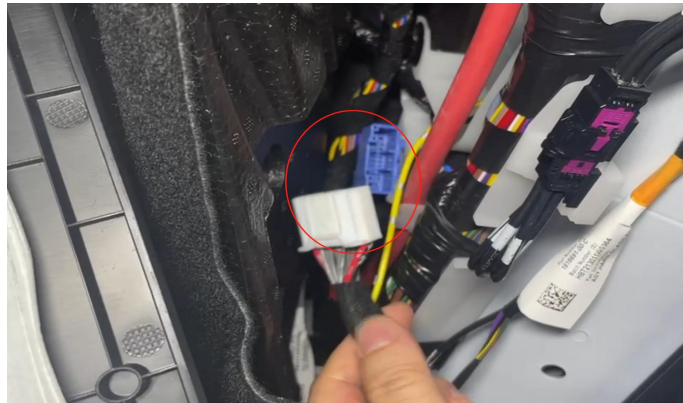
(2) .拆下副驾 A 柱饰板 CAN 线直接与蓝色插座对插 Remove co-pilot's A-pillar trim panel and plug the CAN cable directly into the blue socket
