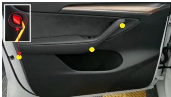
(1).卸下上图三处螺丝 Remove the three screws in the picture above
