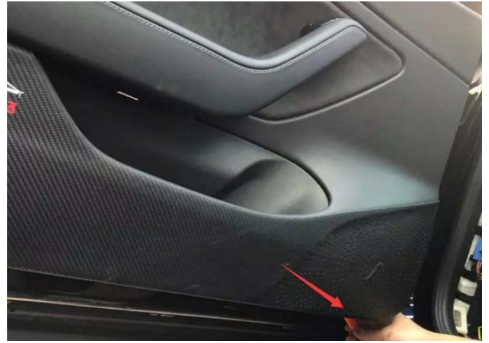
(2). 用撬刀撬右下角 卸下门饰板 Pry the lower right corner with a pry knife to remove the door trim panel
