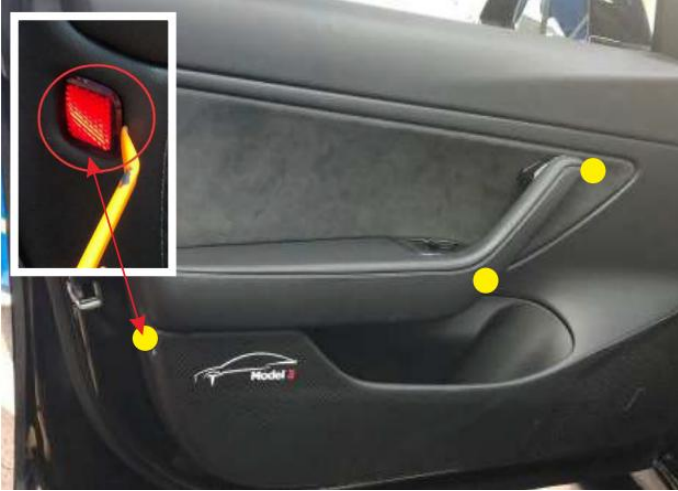
(1). 卸下上图三处螺丝 Remove the three screws in the picture above
