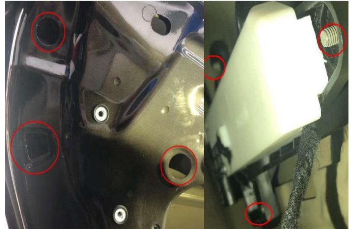
(8).取出上图三颗螺丝，拆下原车把手 Take out the three screws in the picture above and remove the original handlebar
