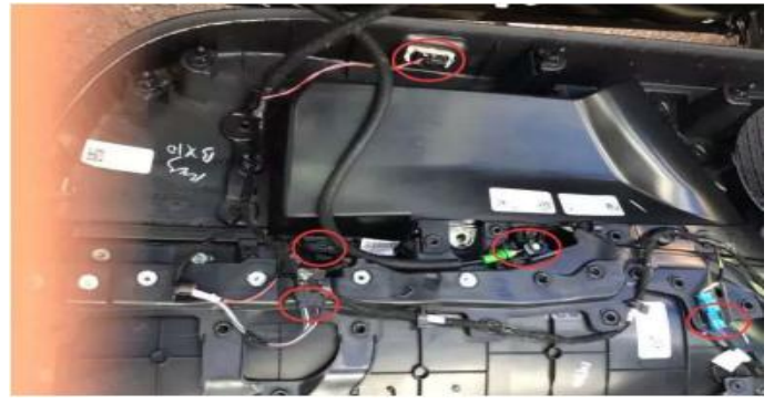
(4).把与盖板相连的插线拔下 拿下盖板 Remove and remove the plug wire connected to the cover plate
