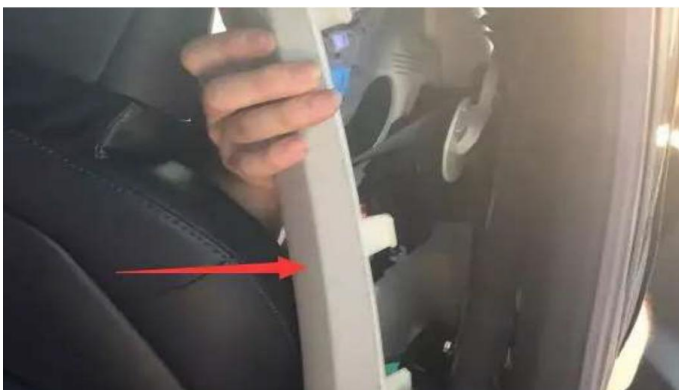
(9).拆下 B 柱上边饰板 用穿线绳将把手线从波纹管穿到车内，线材隐藏在车边沿饰板内 Remove the upper edge panel of pillar B and thread the handle line from the bellows to the inside of the car with the string, the wire is hidden in the edge panel of the car
