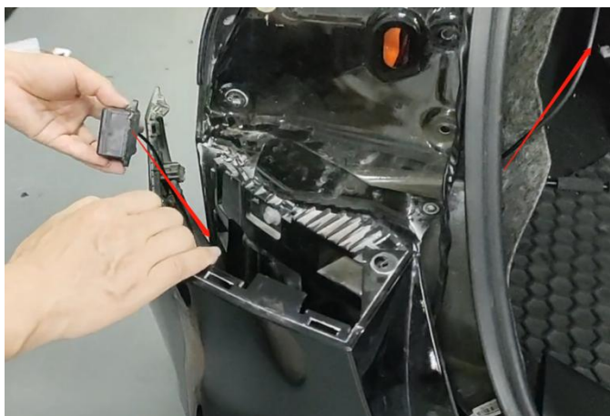
17.把雷达从通风口穿线到后备箱饰板内最后走线到门板上 Thread the radar from the vent to the trim cover of the trunk, and put it to the door panel.
