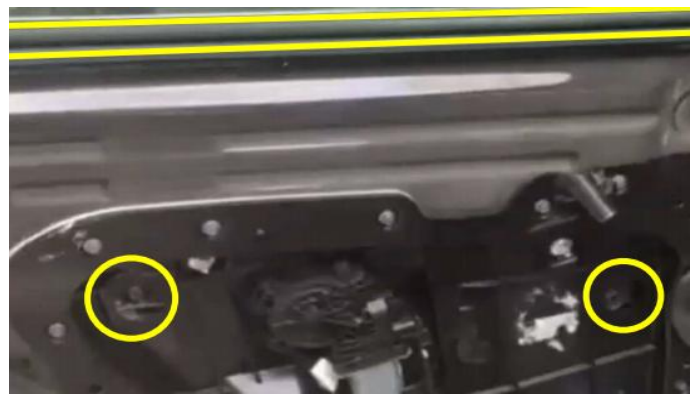
6. 拿出标示处胶条和胶塞把两圆圈内玻璃螺丝拧出就可以直接把玻璃拿出来了 Take out the rubber strip and rubber plug at the mark and unscrew the glass screws inside the two circles to take out the glass directly
