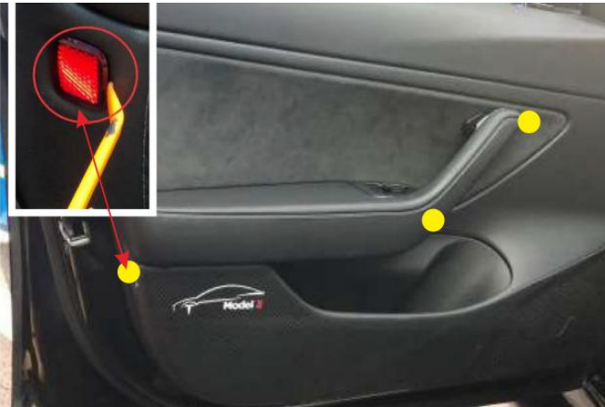
1. 卸下上图三处螺丝 Remove the three screws in the picture above
