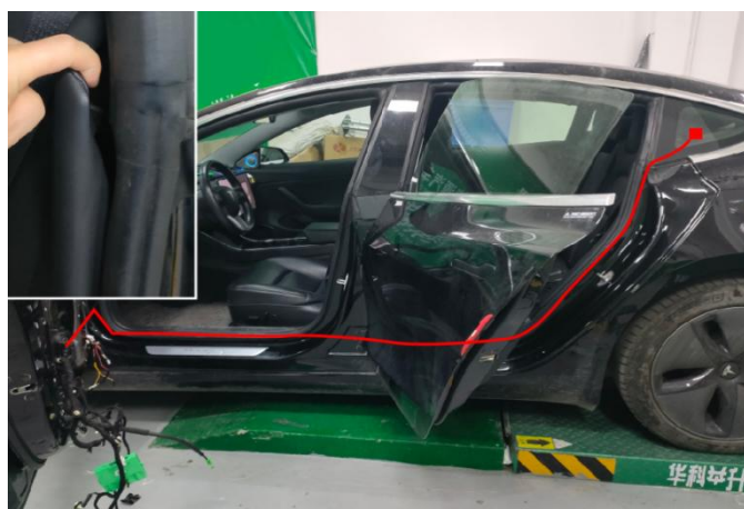
20.自动开门雷达如上图走线到门板上 The wiring of the automatic opening radar.
