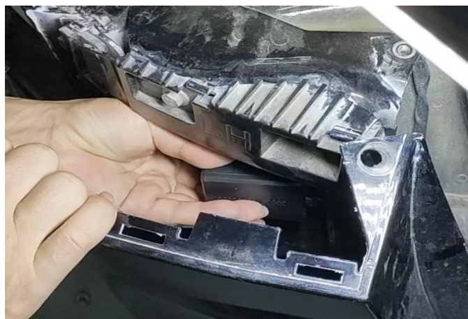
18.把感应器用 3M 胶横着固定, 注意感应器箭头向上朝向车外 Fix the sensor horizontally with 3M tape, pay attention to the sensor, the arrow pointing upwards, and face to rear side.
