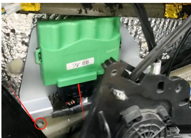
30.总线对插控制盒, 支架背面用 3M 胶固定在门板上 然后在红圈处固定一颗螺丝 The plug of the harness connect to the control box. Paste one 3M sticker on the back, and fixed to the door panel. Fixed one screw at the red circle position.
