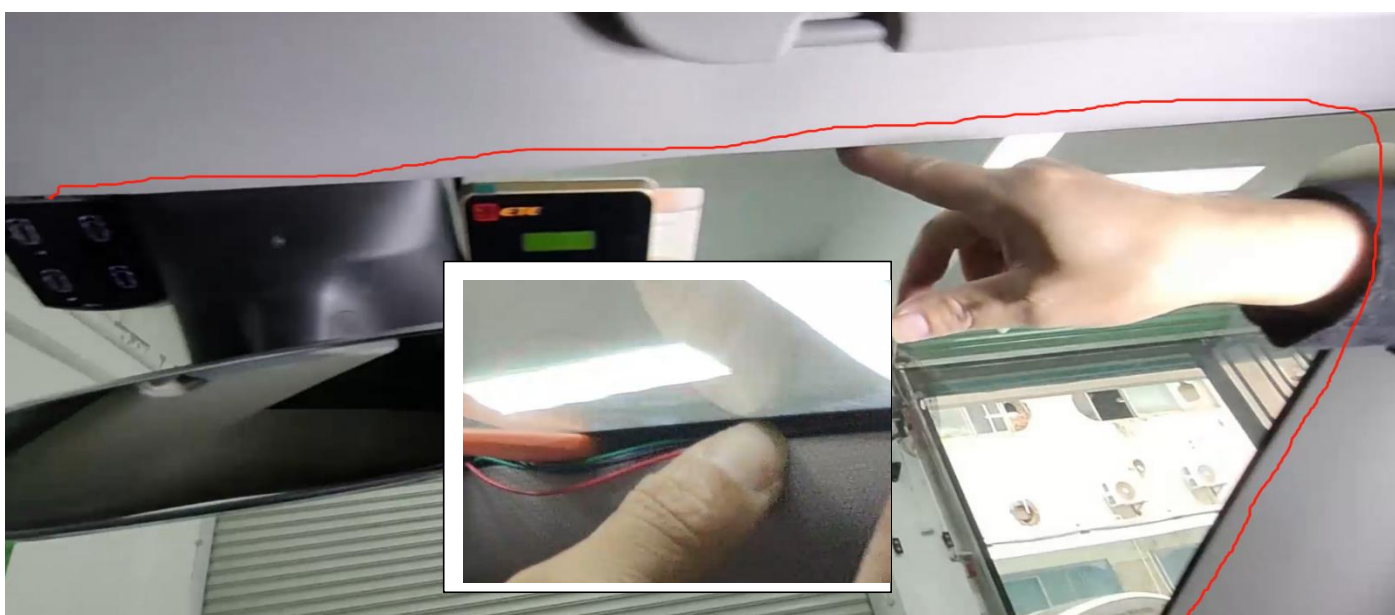
21.把顶蓬开关门按钮用 3M 胶贴在上图位置, 把线材隐藏在饰板缝隙内 Paste the roof switch to the position shown above by 3M sticker. Hide the cable between the trim panel gap.
