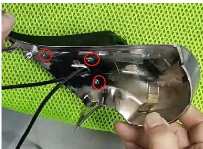
11.把防撞雷达用三颗螺丝固定到盖板上 Fixed the anti-collision to the mirror cover.
