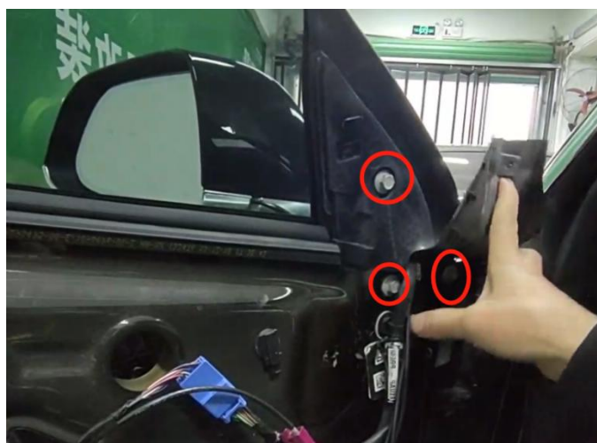
8. 取下后视镜三颗螺丝，拔掉插座取下后视镜 Remove the screws of the Rearview mirror. Unplug the socket and take out the rearview mirror.
