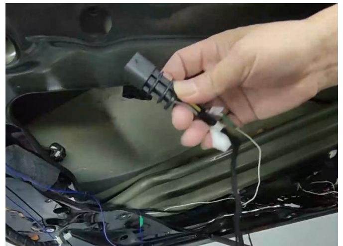
4.电吸插座与原车插头对插 Connect the suction lock to the original socket
