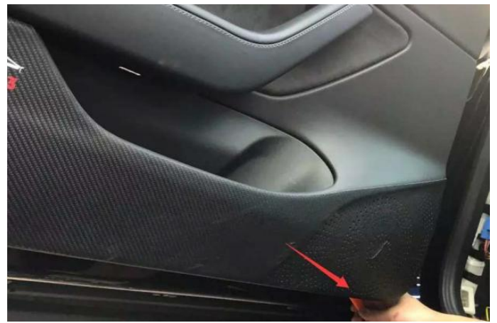
2. 用撬刀撬右下角 卸下门饰板 Pry the lower right corner with a pry knife to remove the door trim panel
