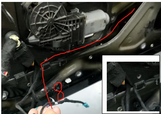
28.八号线如上图走线 No.8 cable wiring.
