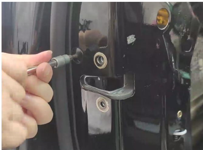
3.取下三颗螺丝安装我司电吸锁，用我司螺丝固定 Take out the three screws and install our suction lock. Fixed with our screws
