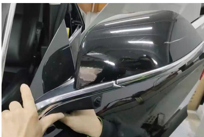
13.把后视镜安装回原车上，对插好原车插头 Install the rearview mirror back to the car, connect the plug.
