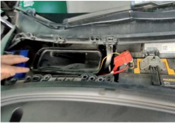
22. 在车前盖电池取电，左边找孔穿线至副驾驶 Take power at the front trunk. Find the hole on the left and threading the wire to the copilot.
