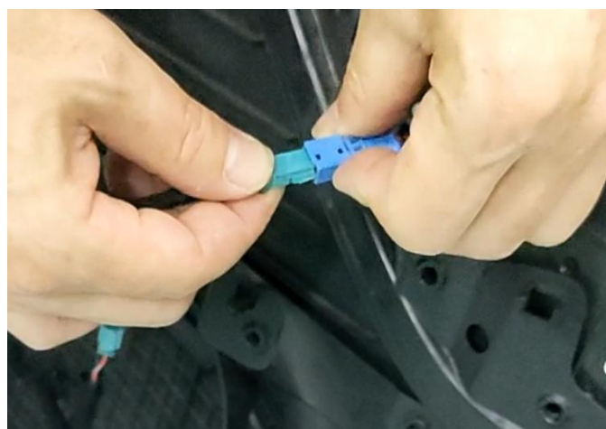
29.八号线转插在门板上 No.8 connect to the door panel.
