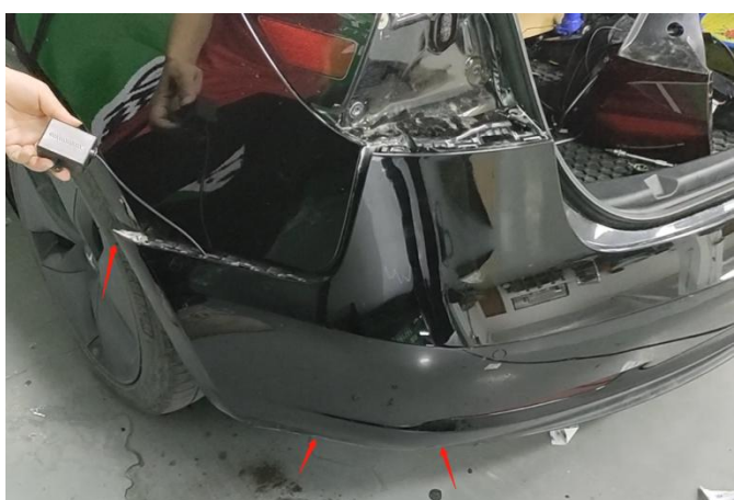
15.拆下三处螺丝和尾灯 Remove three screws and the tail lamp.
