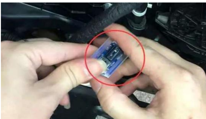
5. 把饰板处如图灯取出来插回去(非常重要) Take out the lamp from the trim plate and insert it back (very important)
