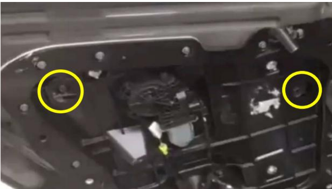
3. 拿出标示处胶条和胶塞把玻璃螺丝对上孔位 Take out the rubber strip and rubber plug at the marking point and align the glass screw with the hole
