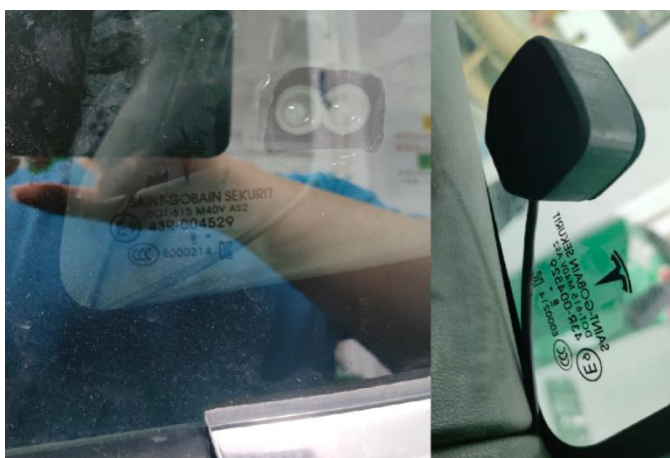
19.把自动开门雷达贴在侧后方玻璃上(贴的靠下一点)Paste the automatic opening radar to the side rear glass.
