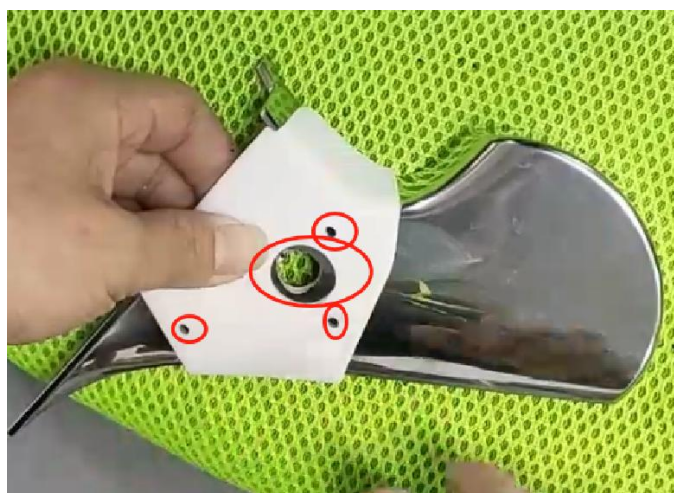
10. 用定位器在盖板开 3 个小孔 1 个大孔 Drill three small hole and a big hole by our cover.
