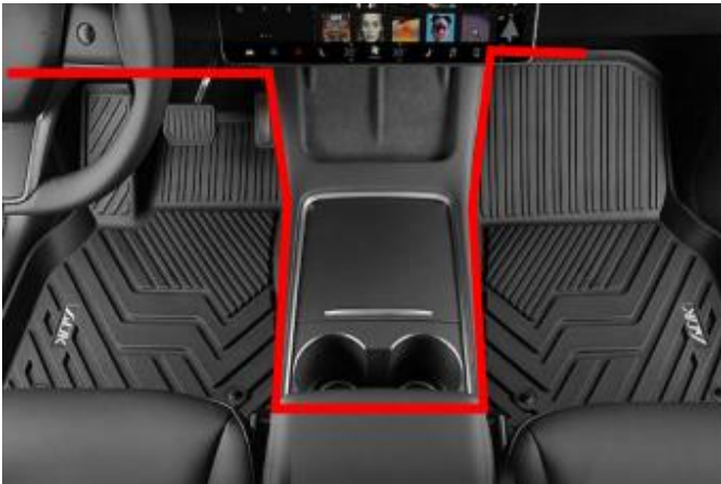
24. 安装主驾智能门，电源线、协议线如上图走线至门板上 Install the driver's intelligent, power wire, signal wire as the wiring shown above.
