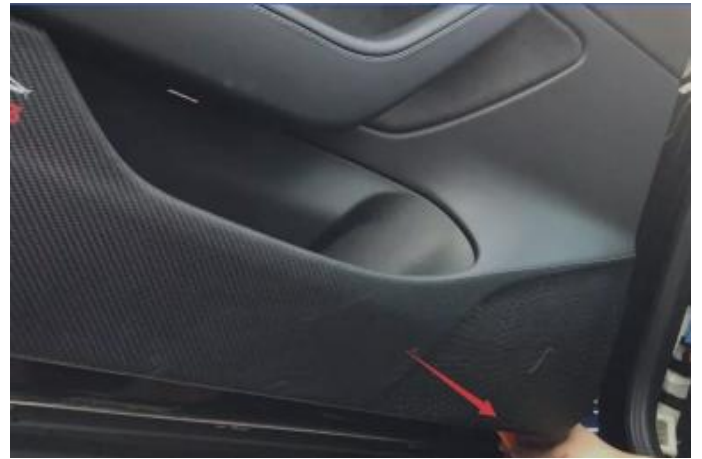
(2) .用撬刀撬右下角 卸下门饰板 Pry the lower right corner with a pry knife to remove the door trim panel
