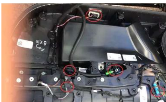
(4) .把与盖板相连的插线拔下 拿下盖板 Remove the plug wire connected to the cover plate and remove the cover plate
