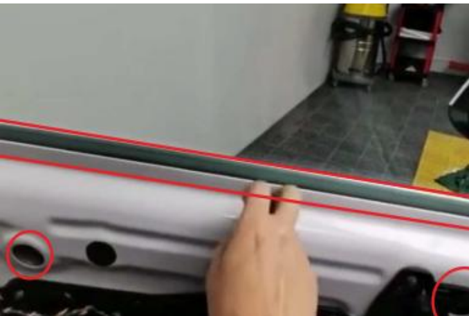
(3) .拿出标示处胶条和胶塞把玻璃螺丝对上孔位 Take out the rubber strip and rubber plug at the marking point and align the glass screw with the hole
