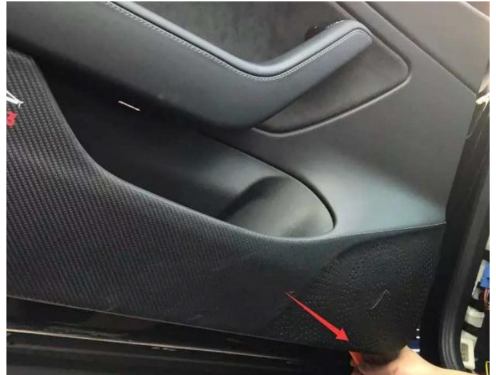
(2) .用撬刀撬右下角 卸下门饰板 Pry the lower right corner with a pry knife to remove the door trim panel
