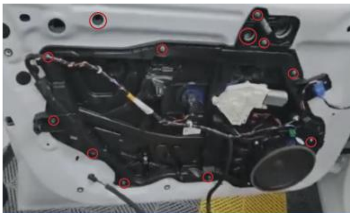
(5) .拔掉所有插头取下标记的所有螺丝拿下饰板 Unplug all plugs, remove all marked screws and remove the trim plate
