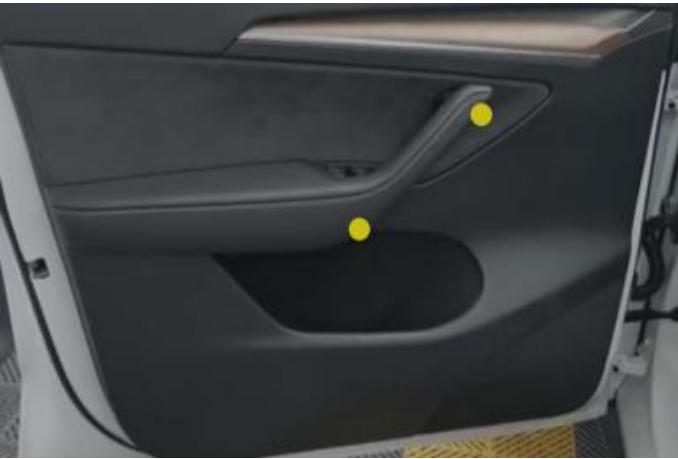
(1) .卸下上图两处螺丝 Remove the two screws in the figure above
