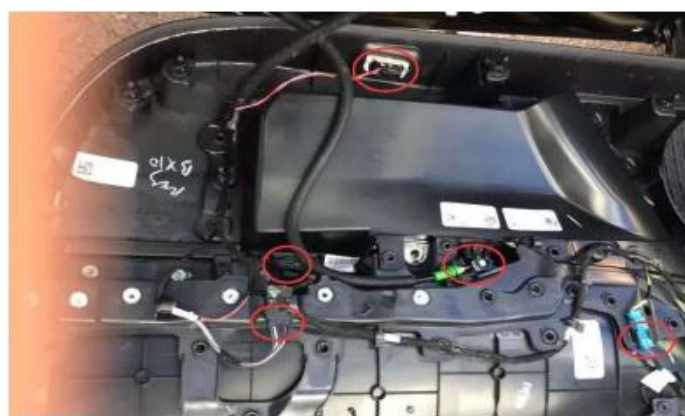
(4) .把与盖板相连的插线拔下 拿下盖板 Remove and remove the plug wire connected to the cover plate
