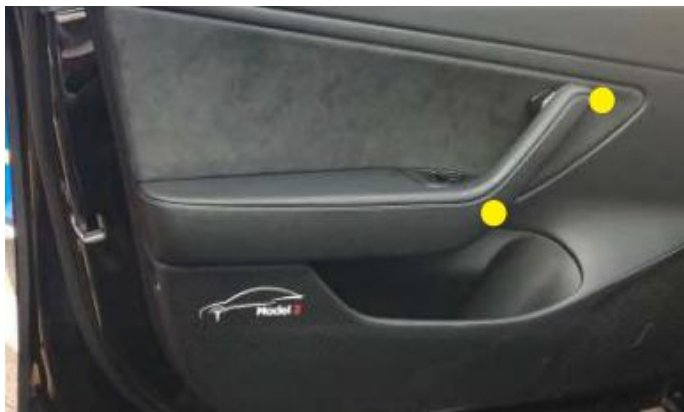
(1) .卸下上图两处螺丝 Remove the three screws in the picture above
