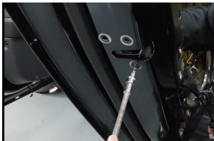
(12).拧好螺丝后 测试车门正常后 即可复原车门 Restore the door after the test door is normal after screwing the screws
