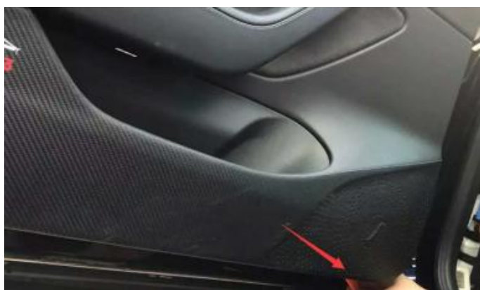
(2) .用撬刀撬右下角 卸下门饰板 Pry the lower right corner with a pry knife to remove the door trim panel
