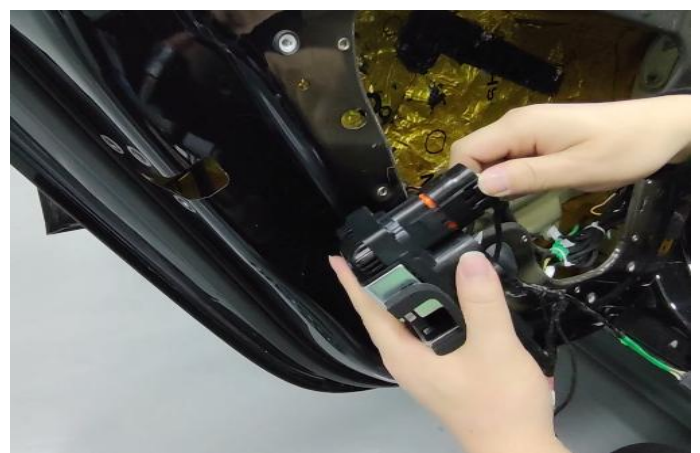
(10).将原车插头和我司智能一体锁连接 connect the plug of the original car with our intelligent integrated lock
