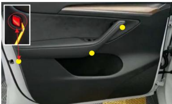
(1) .卸下上图三处螺丝 Remove the three screws in the picture above
