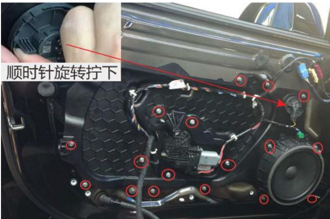
(7).卸下固定饰板上的所有螺丝 Remove all screws from the fastening trim plate
