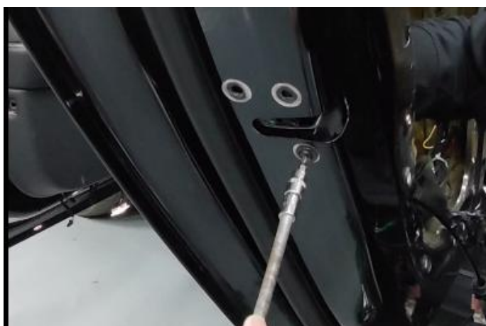
(9) .拧好螺丝后 测试车门正常后 即可复原车门 The door can be restored after the test door is normal after screwing the screws
