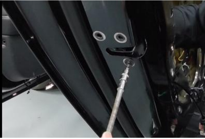
(11) .拧好螺丝后 测试车门正常后 即可复原车门 Restore the door after the test door is normal after screwing the screws
