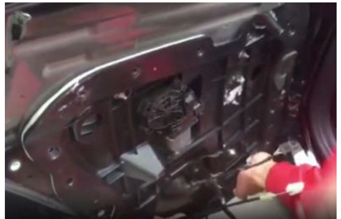
(8).把与固定饰板上连接的所有线取下,用手从固定饰板下端用力往上提的同时往外拉出即可取下饰板 Remove all the wires connected with the fixed plate and pull out the lower plate by hand while lifting the lower end of the fixed plate forcefully
