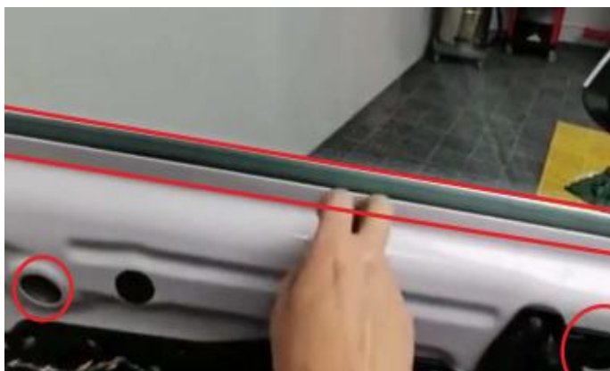
(3) .拿出标示处胶条和胶塞把玻璃螺丝对上孔位 Take out the rubber strip and rubber plug at the marking point and align the glass screw with the hole
