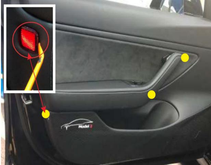
(1) .卸下上图三处螺丝 Remove the three screws in the picture above
