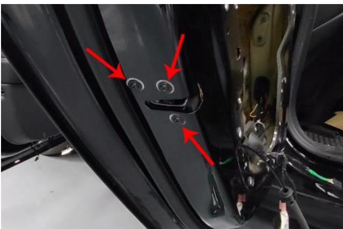
(9).取出上图三颗螺丝,拆下原车锁 Take out the three screws shown above and remove the original lock
