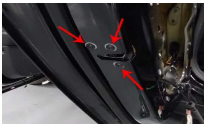
(6) .取出上图三颗螺丝，拆下原车锁 Take out the three screws shown above and remove the original lock
