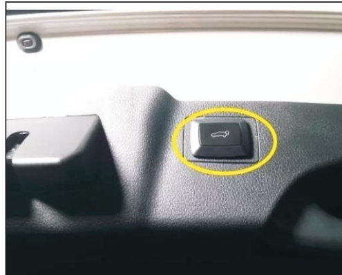
17. At the tail door trim remove square trim punch, install our stern door switch button
