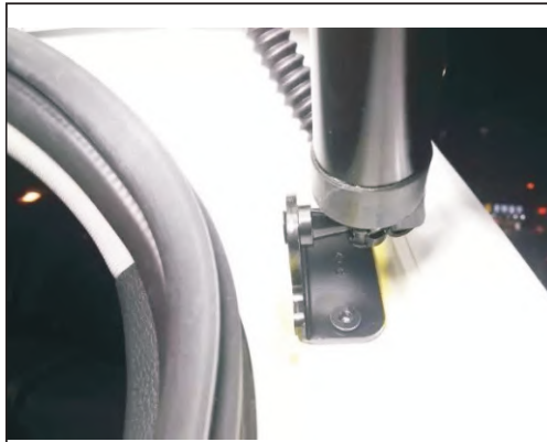
5. Remove the original car right bracket, installation bracket at the lower right, using screws, install the poles
