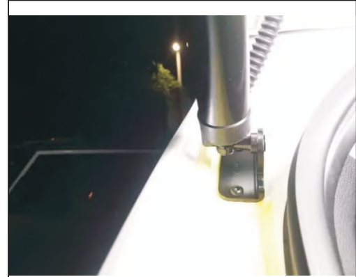
3. Remove the original car bottom bracket, installation, bottom bracket, with screws, install poles (with line down at the end of the poles)
