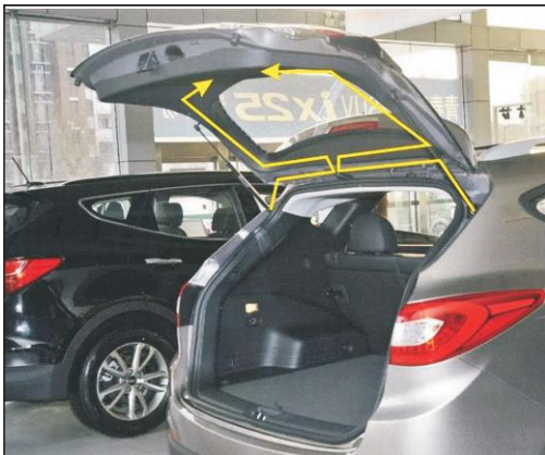
7. Hall line running from the hole through the waterproof rubber plug, go line to end door cover central control box, to thrust control boxes, as shown
