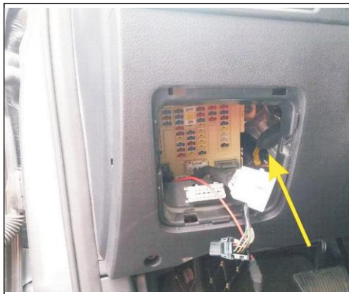
8. Remove the trim at the bottom of the main drive, found the power supply, as shown
