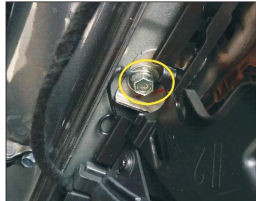
12. Connected to ground
