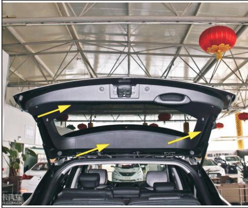
1. Remove the original rear door trim
