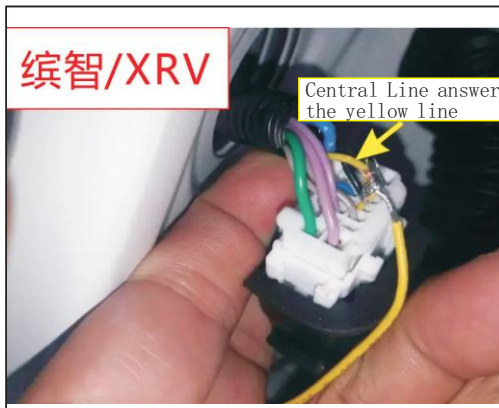
14. Bean wisdom/XRV Central Line connection, count from left to right in the first row fourth hole (pictured)
