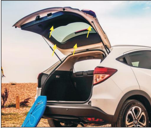
5. The yellow arrow tail door plaque to be removed
