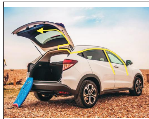
15. The power cord, door control line go line to end cover central control box
