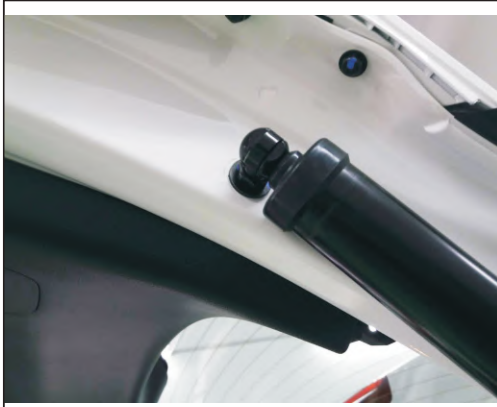
2. In the original car ball head with a gasket installation our poles (poles with line up)
