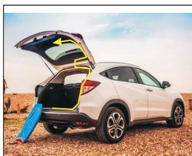
22. Electric door suction line go line to end cover central control box
