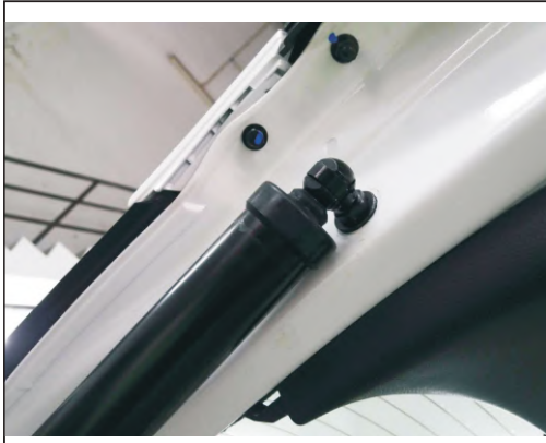
4. In the original car ball head with a gasket installation our poles (poles with line up)
