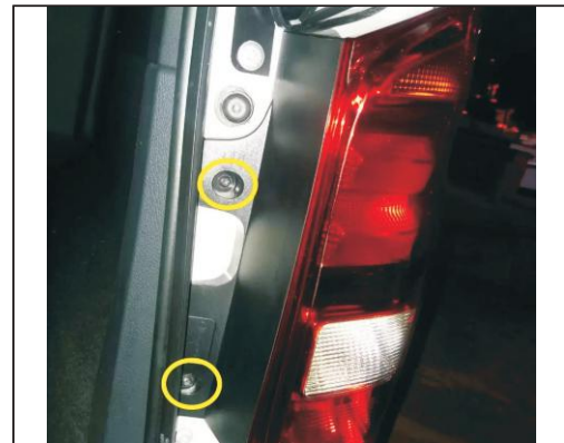
6. The two screws removed within the yellow circle, remove the lights (or steps)
