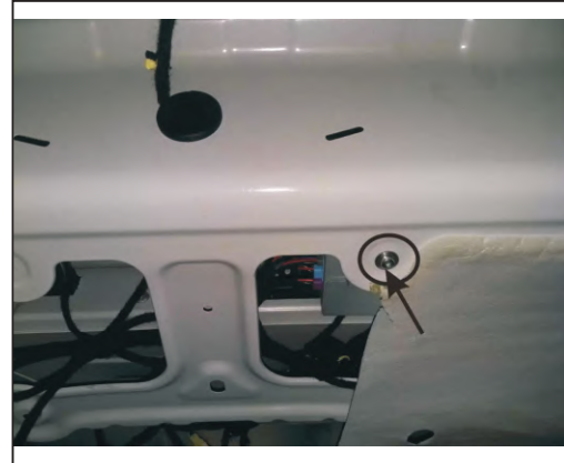
18. Sucked and poles, electric outlet a pair of control box, installation position and control box, use the original car fixed screws, springs and washers
