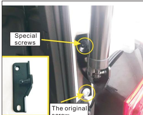
2. Remove the original car right bracket and brace, we lower bracket installation, pay attention to the stent placement, ball head itself, in our screws, the screws with the original car. Note: to be one of the door
