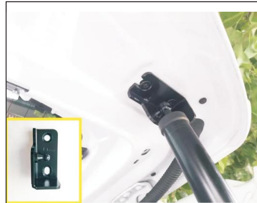
3. Remove the original car right bracket and brace, our upper bracket installation, pay attention to the stent placement, ball head, with our screws
