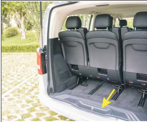
16. Remove the plaque, find the original lock buckle
