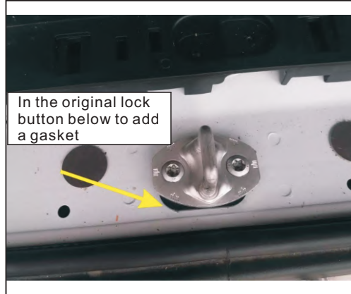
17. Remove the original lock buckle, in the original lock button below to add a gasket
