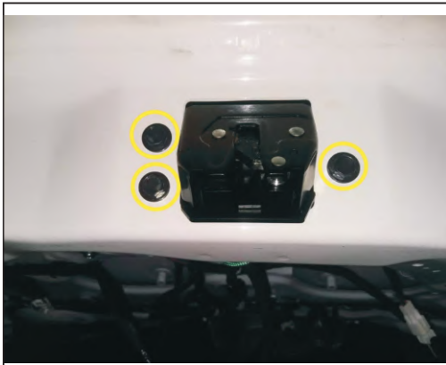
13. Remove the original car door lock, installed on our electric lock, use the original car screws
