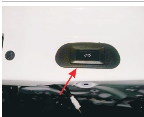
20. Remove the original car trim, install our stern door keys
