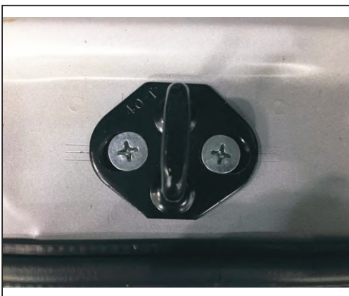
11. Remove the original lock buckle, installing special lock ring, with the original screw fixation
