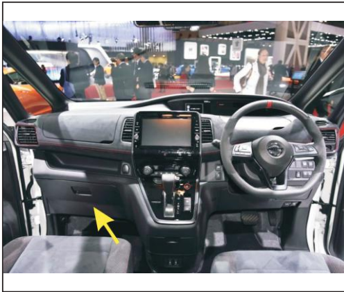
5. Remove the trim at the bottom of the co-pilot to find the original car power supply
