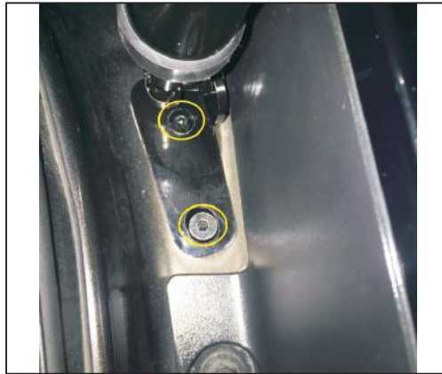
3. Remove the original car right bracket, installation we lower bracket (ball head) within the body, with screws
