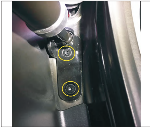
2. Remove the original car bottom bracket, installation we lower left bracket (ball head) within the body, with screws
