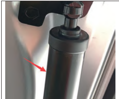
9. Installation of left and right electric pole is completed
