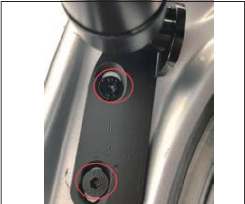
7. Remove the left lower bracket of the original car and install the bracket of our company. Fix it with our company's screw.
