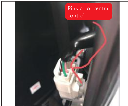
12. Connect the central control wire to the B-pillar
