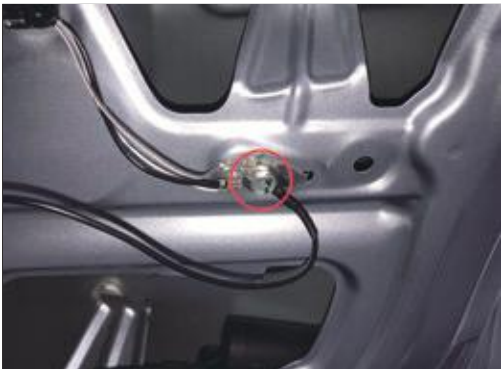
11. Remove the trim board at the right side of the rear tail, find the connection screw of the original car, and connect it to the ground wire of our company.
