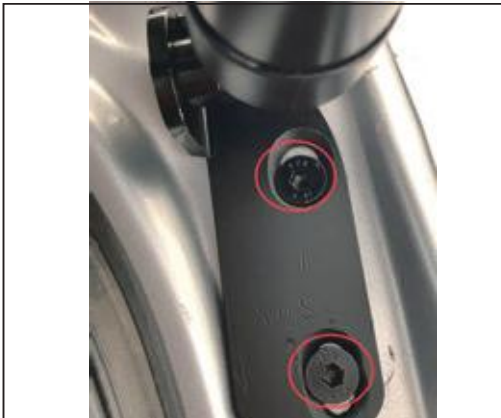
8. Remove the right lower bracket of the original car and install the bracket of our company. Fix it with our company's screw.
