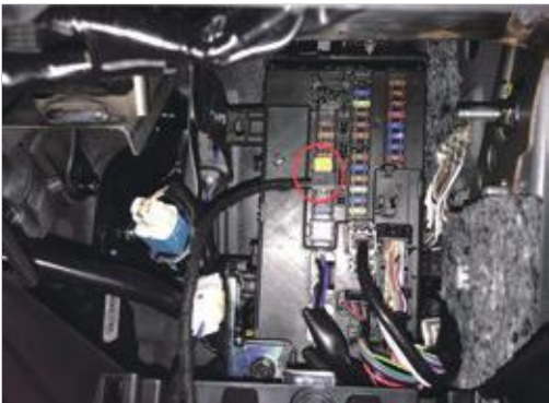
10. Draw electricity from the original car driver compartment
