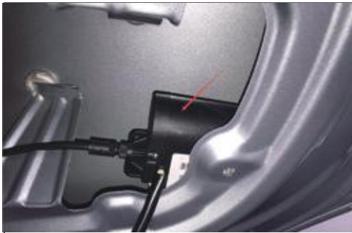
14. Remove the electric suction lock of the original car, install the electric suction lock of our company and fix it with screw
