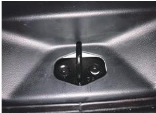
16. Remove the lower lock ring of the original car, install the lower lock ring of our company, and fix it with our company's screw.
