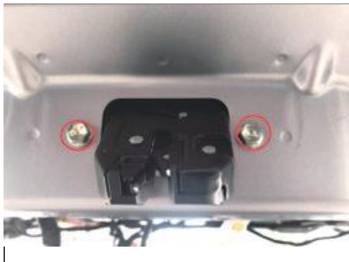
14. Remove the electric suction lock of the original car, install the electric suction lock of our company and fix it with screw
