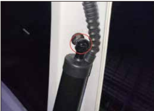
4. Install our electric pole with the original car ball mount (left and right alike)
