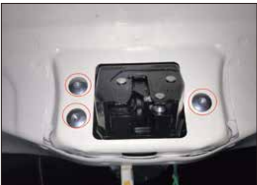
10. Remove the original locks and install our electric suction lock fixed with screws
