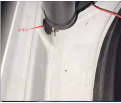
2. Remove the original car lower ball mount and install our inclined ball mount.
