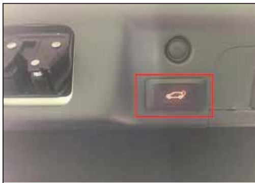
12. Punch holes in the trunk of the original car to install the tailgate switch
