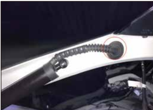
5. Punch holes at this position on the original car and install the wiring of the electric pole.
