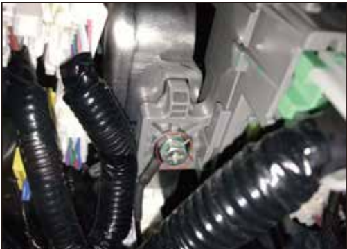
7. Grounded under the original car driver compartment
