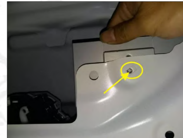
16. Control box installation position, fixed it with our screws, meson and gasket.
