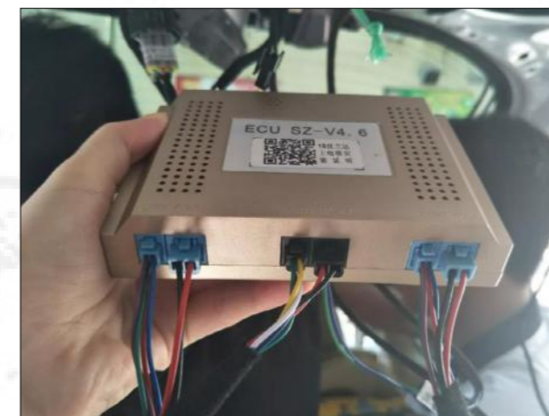
15. According to the color of socket, insert the plugs into the control box.
