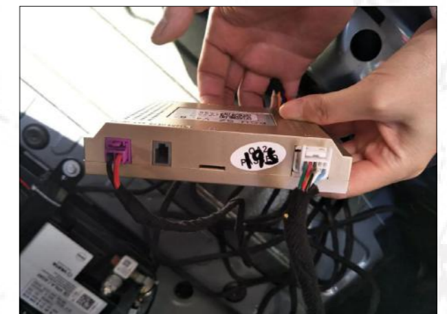
15. According to the color of socket, insert the plugs into the control box.
