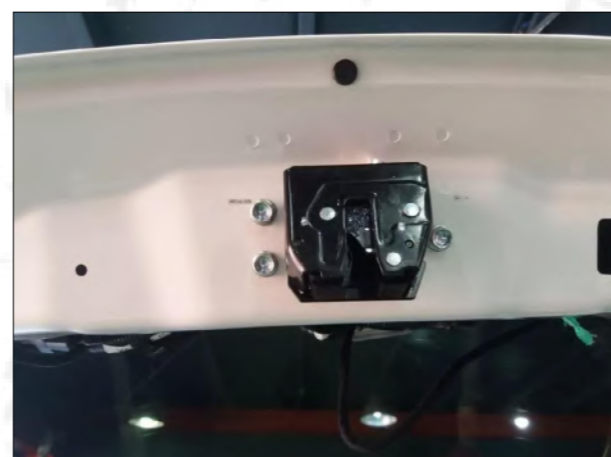
12. Remove the original door lock, then install our upper suction lock and fix it with the original car screws.
