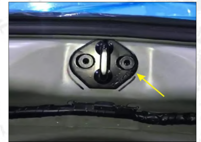
14. Remove the original car locks and place 2 shims or 4 shims under each lock ring hole.
