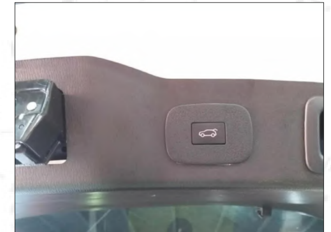
17. Punch a hole on the trim panel. Install our tailgate switch button and restore the trim panel.
