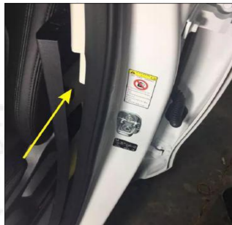
9. Disassemble the trim panel at the main driving belt B-pillar and find the central control line.
