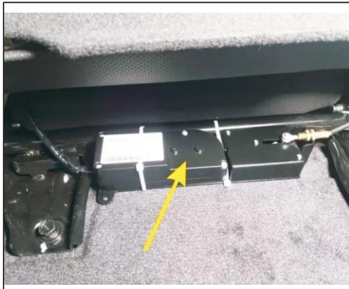
15. Electrical installation location, with our company 3 m glue and cable tie
