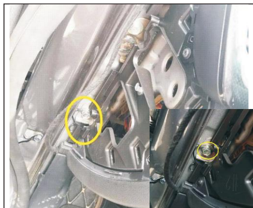
10. In the main drive side trim will be removed, connect the ground wire
