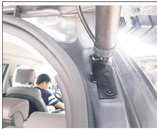
4. Remove the original car right bracket, installation bracket at the lower right, using screws, install our poles
