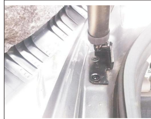
3. Remove the original car bottom bracket, installation, bottom bracket, with screws, install the poles
