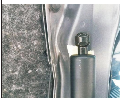
2. Remove the original car poles, ball head installed our poles with the original car
