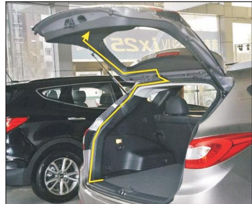
16. The electric door suction line go line to end cover central control box, for our control box
