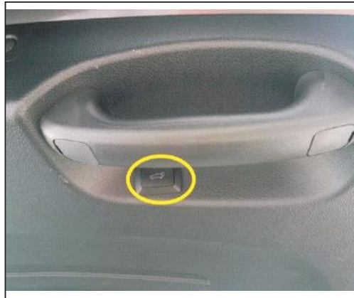
18. In the original rear door trim punch, install our stern door keys
